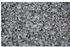
Difficult Materials High F.M., crushed, angular
