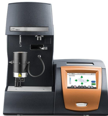
Thermogravimetric analysis to measure the CH consumption
